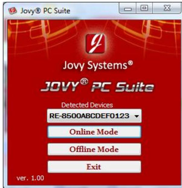
After clicking on Online Mode button, a message “*USB IS CONNECTED*” will appear on LCD and user will be able to control **RE-8500** from PC.
